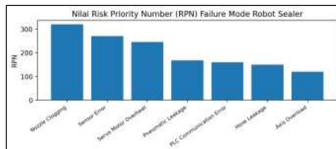
Gambar 3. Nilai RPN Failure Mode Robot Sealer
