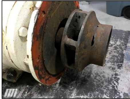
Gambar 1. Impeller Ejector Pump Korosi
