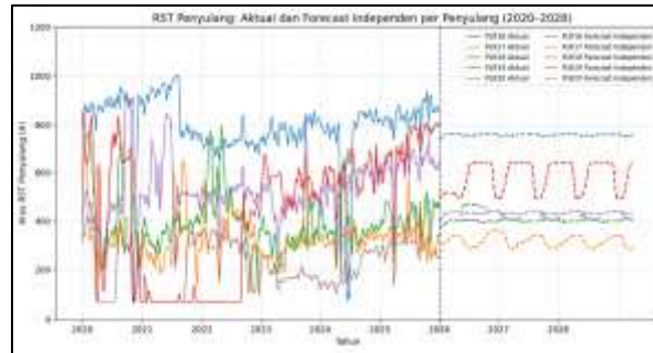
Figure 6. Historical and forecasted daily RST load profiles of feeders PLR16–PLR21 from 2020 to 2028
