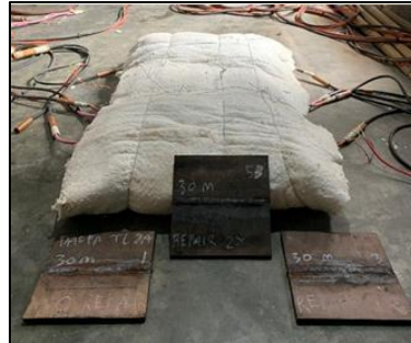
Gambar 2. Proses Post-Weld Heat Treatment (PWHT)
